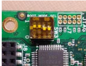
Figure 3: BOOT MODE selection Switch Position
