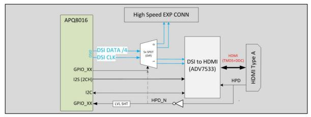
The 96Boards specification calls for a MIPI-DSI to be present on the High Speed Expansion Connector. A minimum of one lane is required and up to four lanes can be accommodated on the connector.
