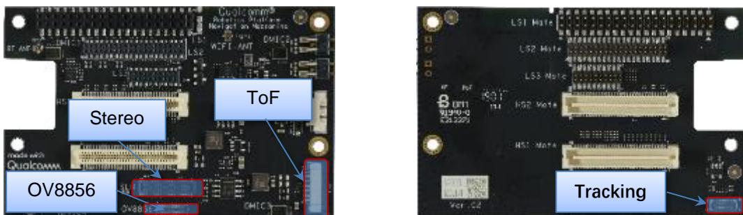
The sensor ID changes depending on the number of camera sensors connected simultaneously.
