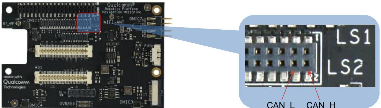
1. Connect CAN\_L and CAN\_H for loopback test.
