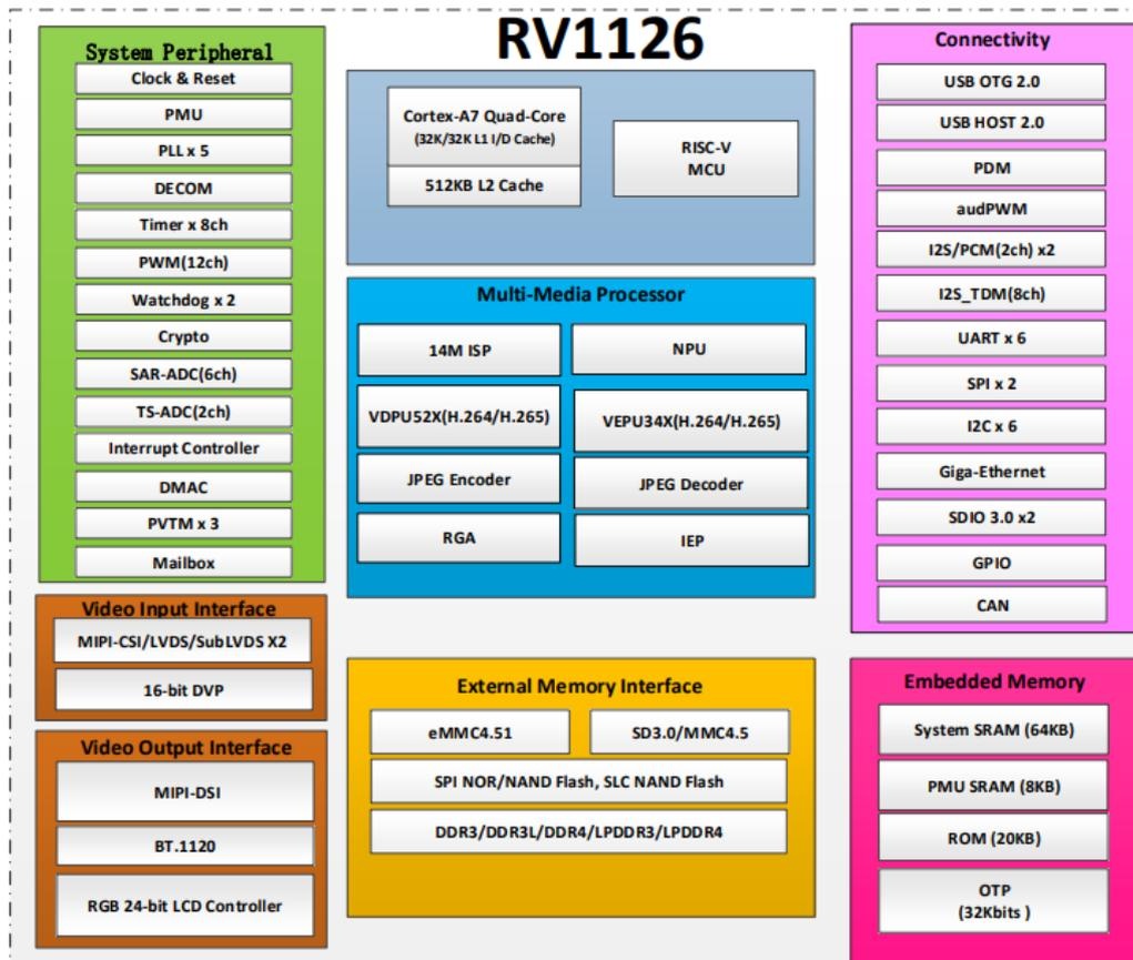
Fig.1-1 Block Diagram
