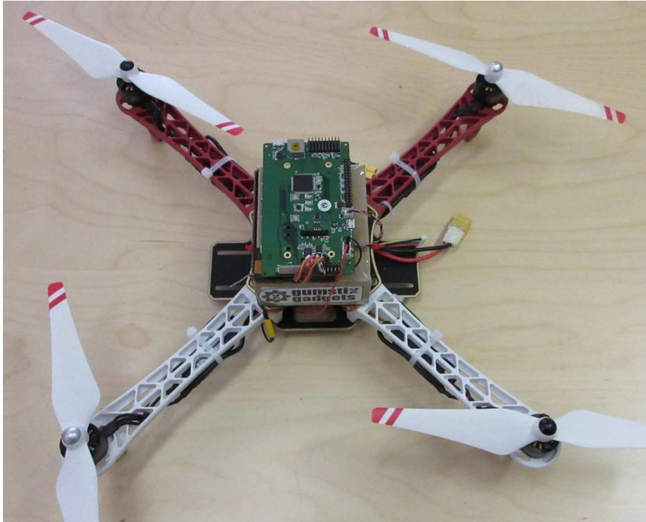
Figure 4: AeroCore 2-based Quad-rotor MAV
