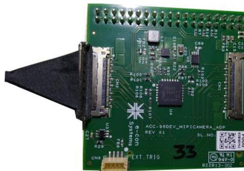
**Figure 12: Unlocking Position of Cable on Base Board CN2 Connector**
