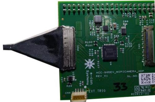
**Figure 13: Locking Position of Cable on Base Board CN2 Connector**
