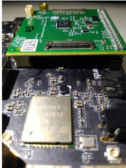
**Figure 8: ROCK960 Development Board with e-CAM50\_CU96 Base Board**
