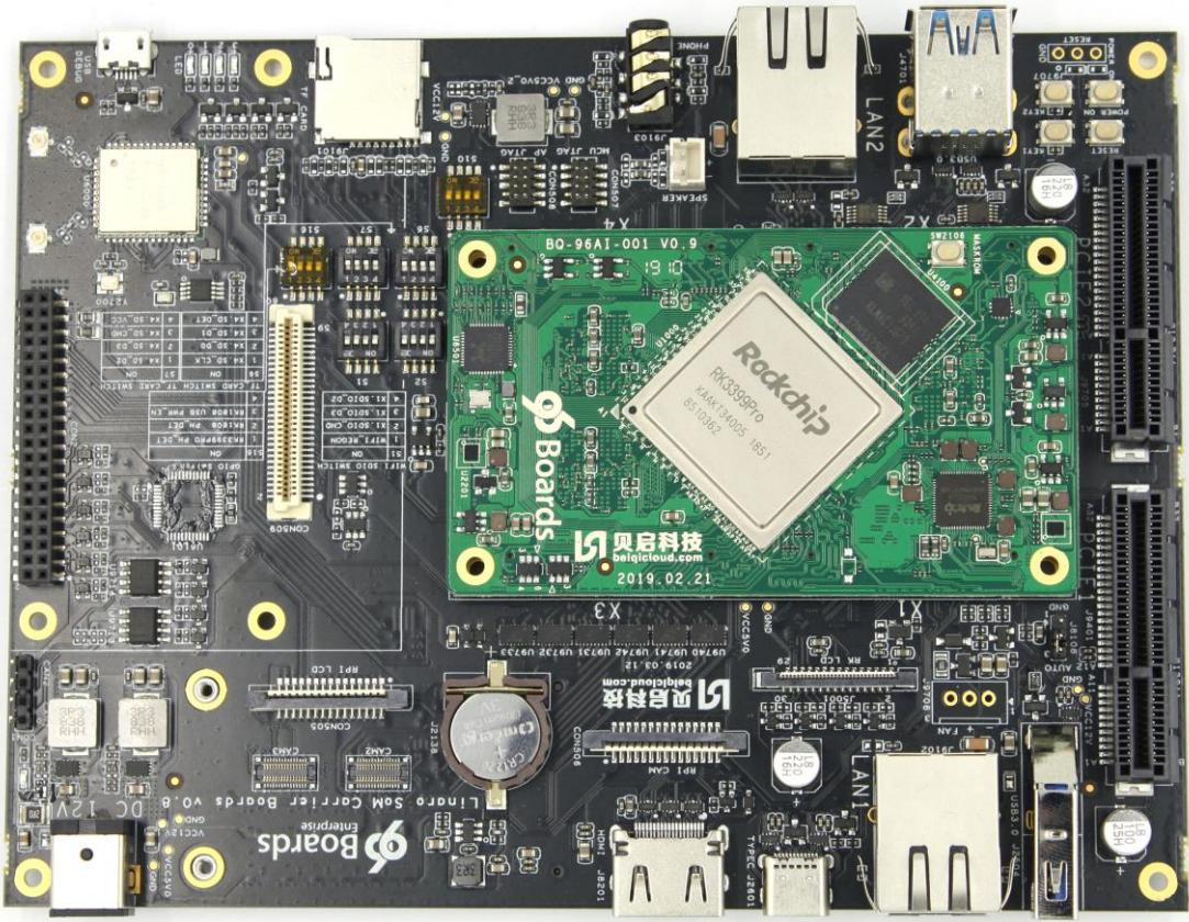
The following figure shows the use of TB-96AI RK3399Pro SOM on the Carrier board.
